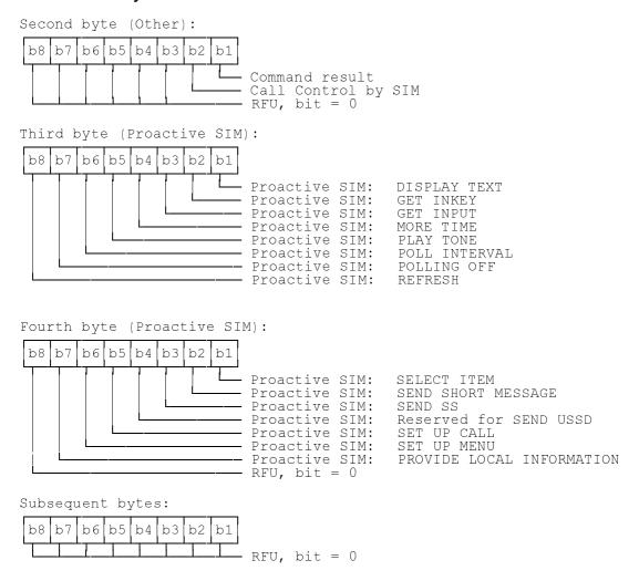
RFU bits, and all bits of subsequent bytes, are reserved to indicate future facilities. A SIM supporting only the features of SIM Application Toolkit defined here shall not check the value of RFU bits.
